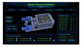
Mineral sizer can be fully automated to ensure continuous optimal performance, matched with a PLC control system for remote automatic control and monitoring, overload protection and other functions, providing a safer working environment.
