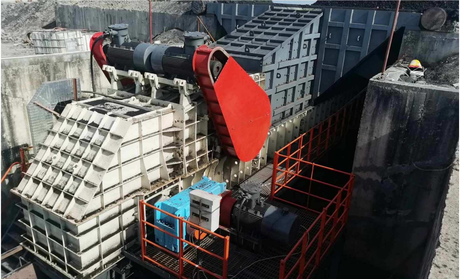
1000TPH/SET PRIMARY FEEDER BREAKER/TOTAL 2 SETS/RAW COAL/INDONESIA
